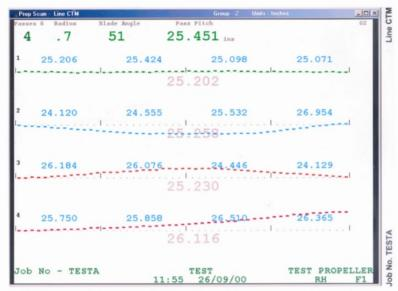
This line graph is an actual screenshot of the Prop Scan system that the technicians use to repair your prop. The top line represents a properly repaired/tuned prop. The others are typical of traditionally repaired props. Notice the belly and collapsed middle which causes slippage. The bottom 3 props are wasting fuel.
